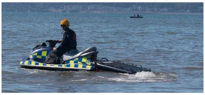
The Jet Ski Rescue Board is an inflatable board that is designed to be attached to the back of a jet ski to aid rapid response and rescue of casualties. It is attached by a towing 'D' ring and two other 'D' rings which are located at the front of the inflatable board.
